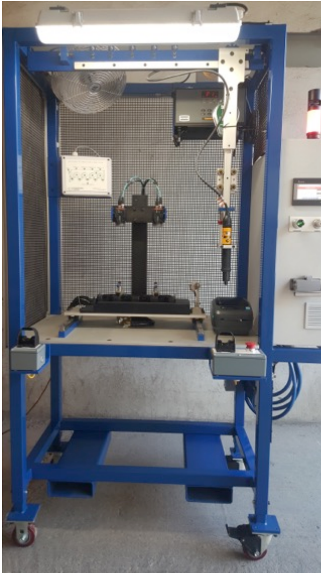
CONMET: Lock Carrier Torque & Vision Station
