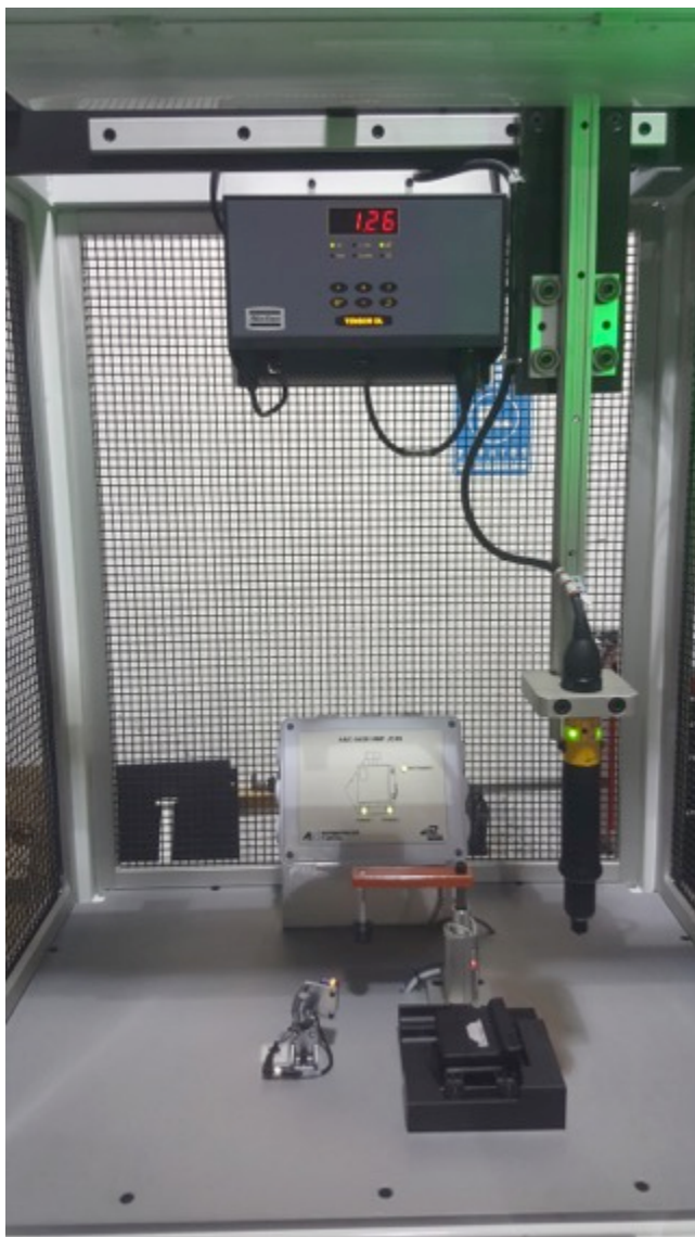
GRUPO ANTOLIN: Assembly Fixture for SGW Module
