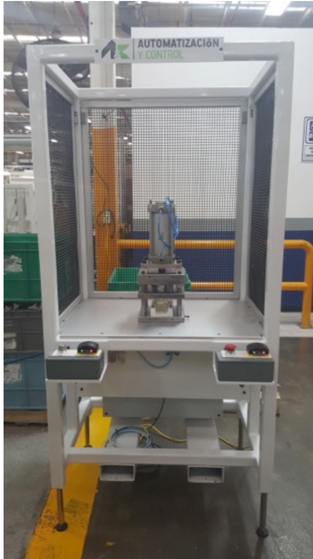
IACNA: Personal Lamp Punch Press
