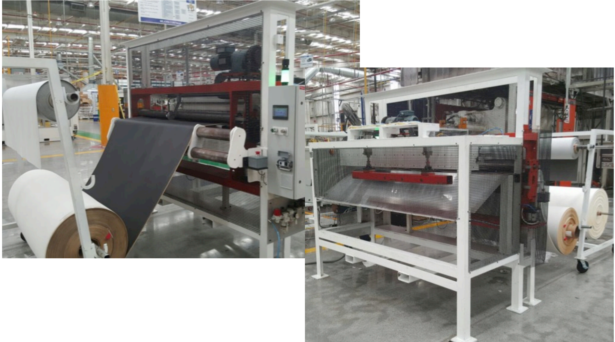
IACNA: Fabric Cutting Station
