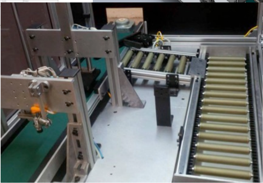
VESUVIUS: Nozzle Identification Vision System Station
