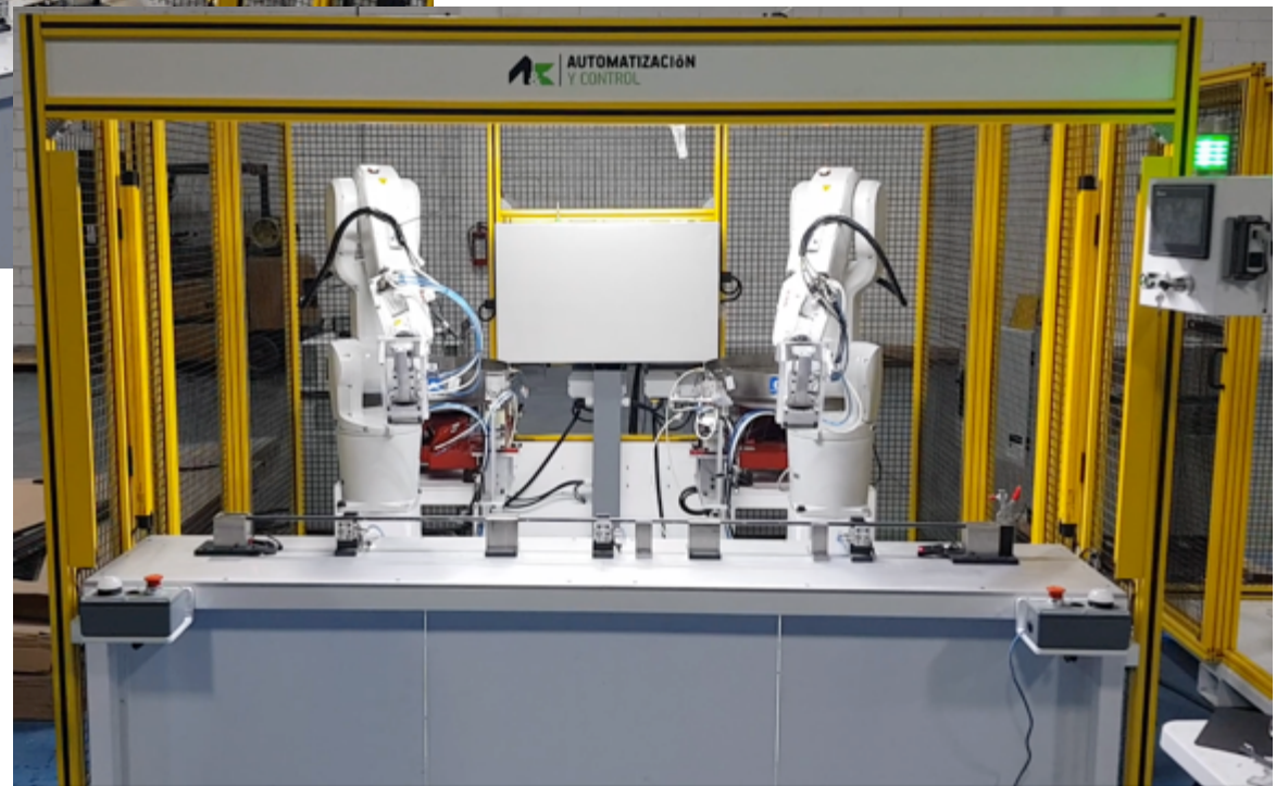
MAGNA: Frt/Rear Door Assembly Station
