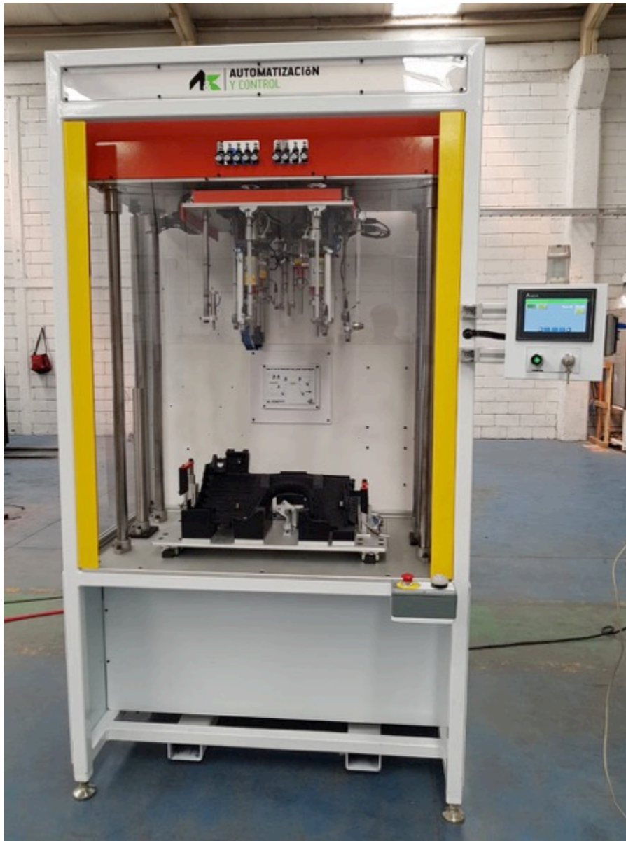
ANTOLIN: CO Cap Hider Ultrasonic Welding Station
