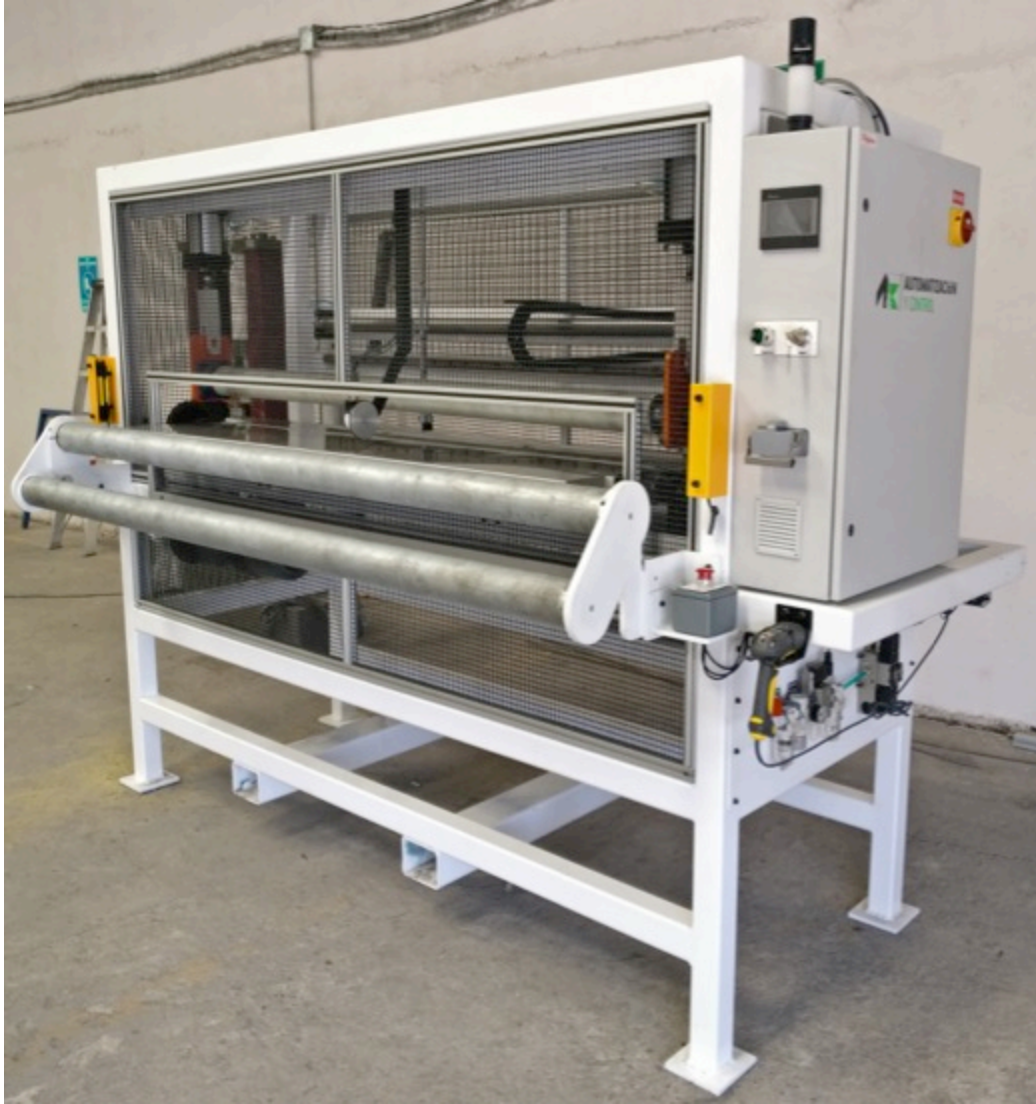
IACNA: Fabric Cutting Station
