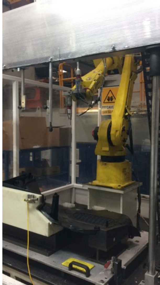
MAGNA: Quarter Reinforcement Welding Station
