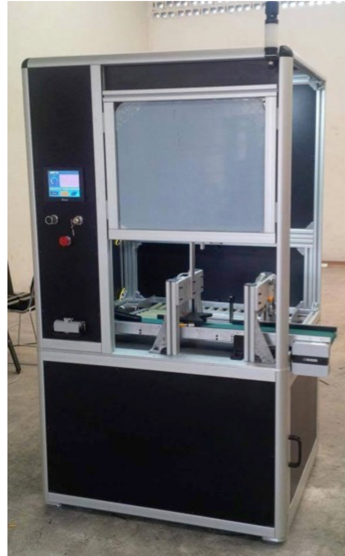
VESUVIUS: Nozzle Identification Vision System Station
