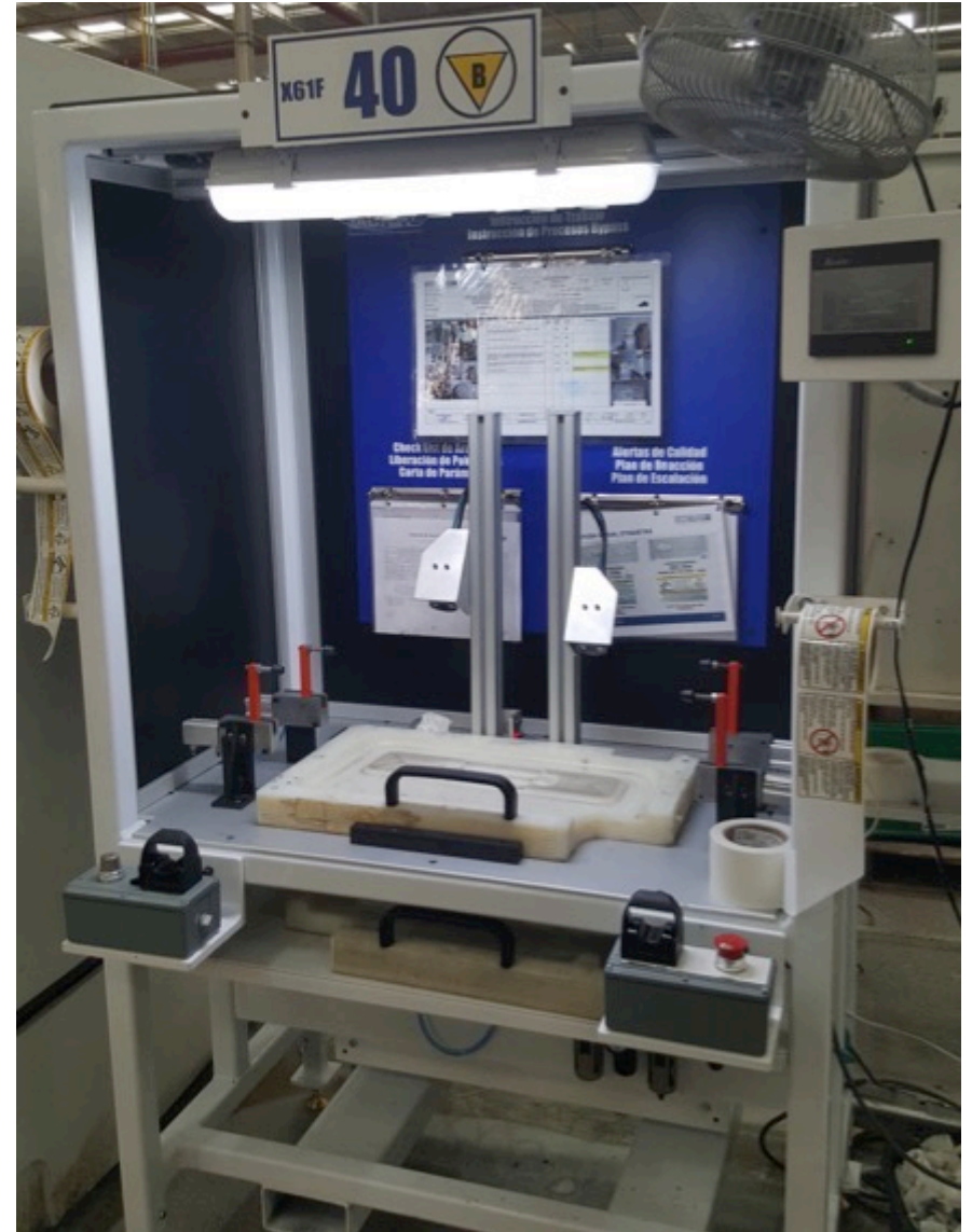
IACNA: Sunvisor Labels Vision Sensor Station
