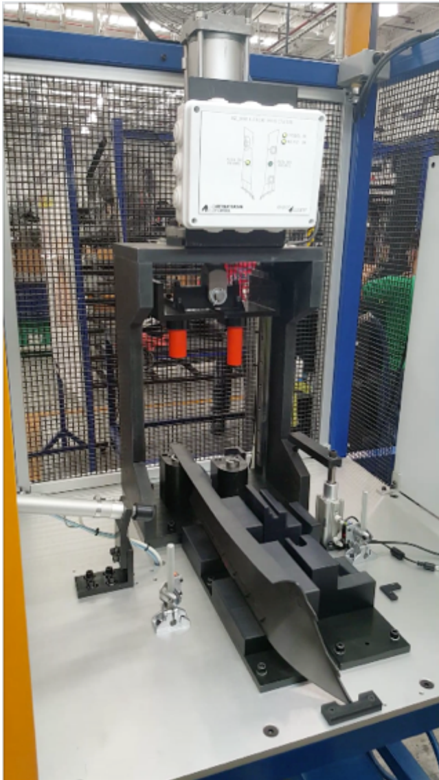
CONMET: Lock Carrier Torque & Vision Station
